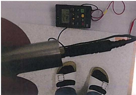
Fig.3 Ascertaining the earth-derivative resistance R_g
